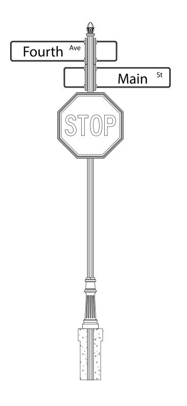
COMPLETE UNIT SHOWN WITH 2' BELOW GRADE BURIAL. FOUNDATION SHOULD BE DESIGNED TO MEET LOCAL CODES AND THE REQUIREMENTS OF SOIL CONDITIONS. DRAWING FOR INFORMATION ONLY, NOT INTENDED FOR CONSTRUCTION PURPOSES.
