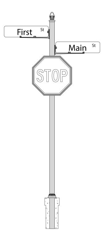
NOTES: COMPLETE UNIT SHOWN WITH 2' BELOW GRADE BURIAL. FOUNDATION SHOULD BE DESIGNED TO MEET LOCAL CODES AND THE REQUIREMENTS OF SOIL CONDITIONS. DRAWING FOR INFORMATION ONLY, NOT INTENDED FOR CONSTRUCTION PURPOSES.
