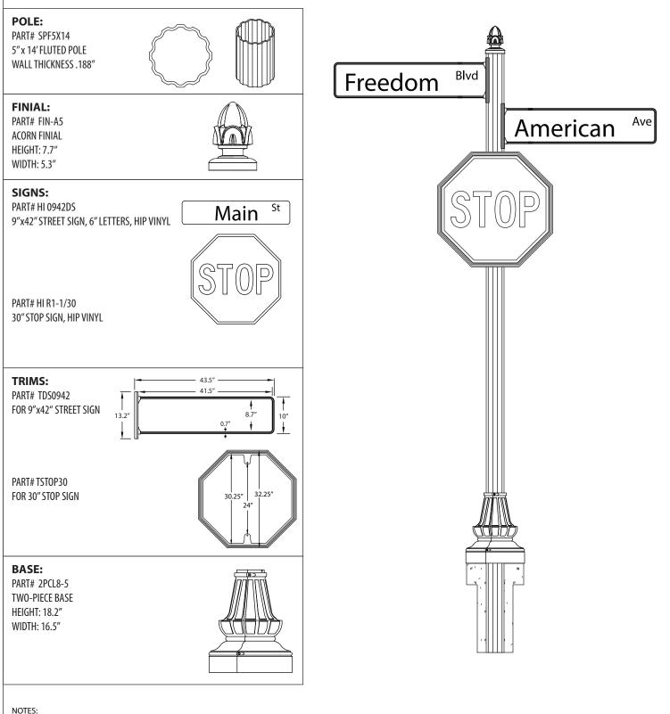
COMPLETE UNIT SHOWN WITH 2' BELOW GRADE BURIAL. FOUNDATION SHOULD BE DESIGNED TO MEET LOCAL CODES AND THE REQUIREMENTS OF SOIL CONDITIONS. DRAWING FOR INFORMATION ONLY, NOT INTENDED FOR CONSTRUCTION PURPOSES.
