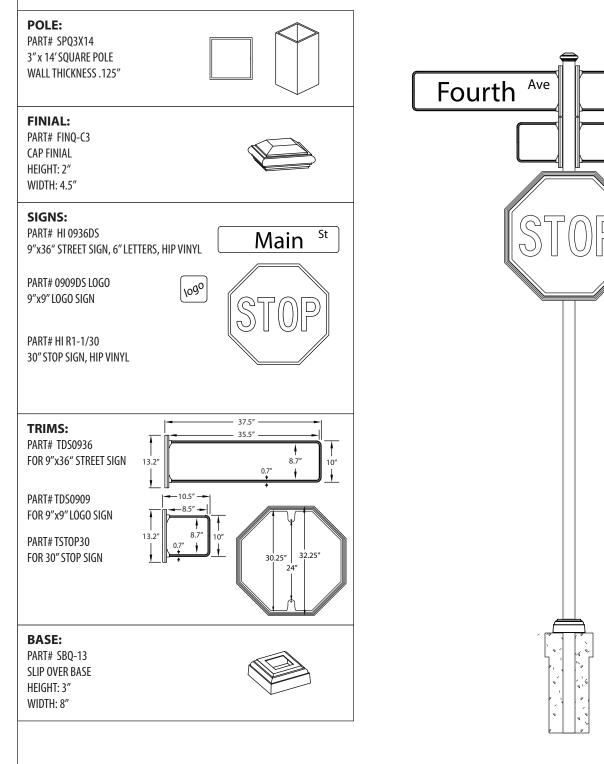
COMPLETE UNIT SHOWN WITH 2' BELOW GRADE BURIAL. FOUNDATION SHOULD BE DESIGNED TO MEET LOCAL CODES AND THE REQUIREMENTS OF SOIL CONDITIONS. DRAWING FOR INFORMATION ONLY, NOT INTENDED FOR CONSTRUCTION PURPOSES.
