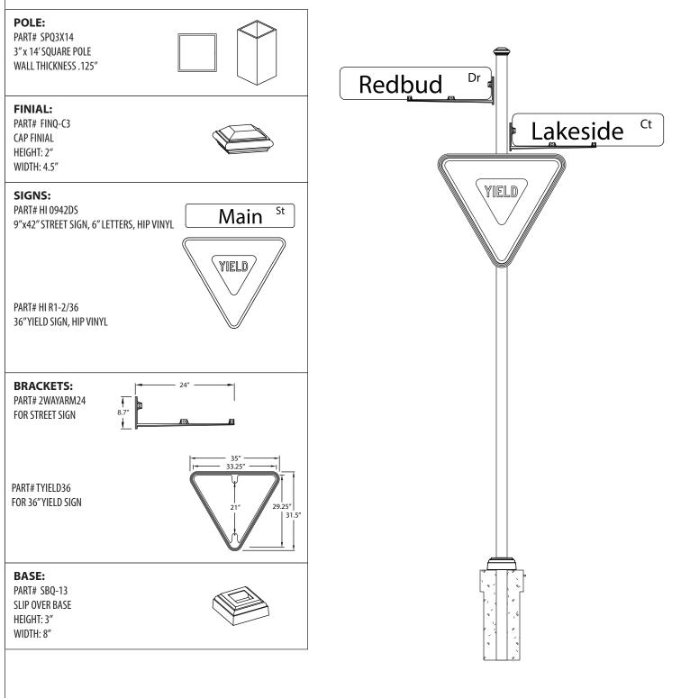
NOTES: COMPLETE UNIT SHOWN WITH 2' BELOW GRADE BURIAL. FOUNDATION SHOULD BE DESIGNED TO MEET LOCAL CODES AND THE REQUIREMENTS OF SOIL CONDITIONS. DRAWING FOR INFORMATION ONLY, NOT INTENDED FOR CONSTRUCTION PURPOSES.
